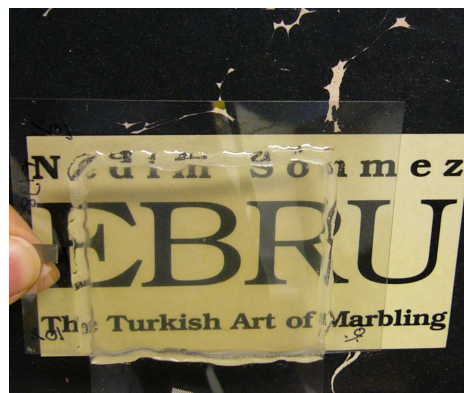
Figure 1. Pictures of SmA PDLCs in an opaque state (top) and in a transparent state (bottom) on 2.5" x 2.5" PET substrates. No voltage is applied to maintain optical states.
