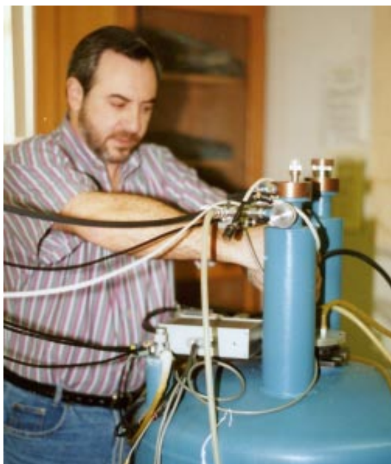
Prof. Finotello tunes the NMR probe to increase its sensitivity to the confined film's behavior.
